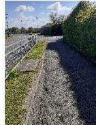
The dropped kerb in front of the school gates is higher than the recommended amount (25mm). Contact can be made with the local council for this to be rectified.
